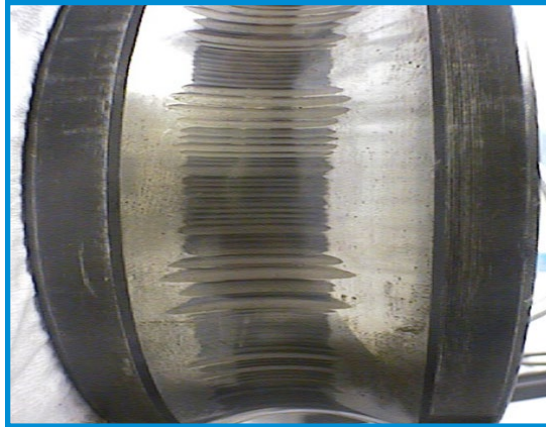
Electrical Damage: Fluting
