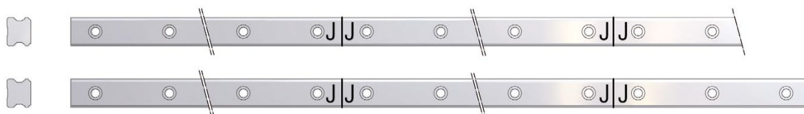
Figure 3.6 Marking of jointed rails
