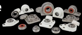
NTN's Sentinel Series is a premium line of corrosion-resistant mounted ball bearing products developed for the harsh conditions of the food & beverage industry. The entire Sentinel Series line features insert bearings constructed from 440C stainless steel with integral bearing seals.
