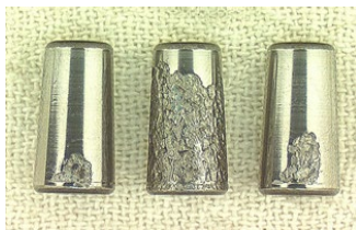
Figure 5: Excessive Axial Preload
