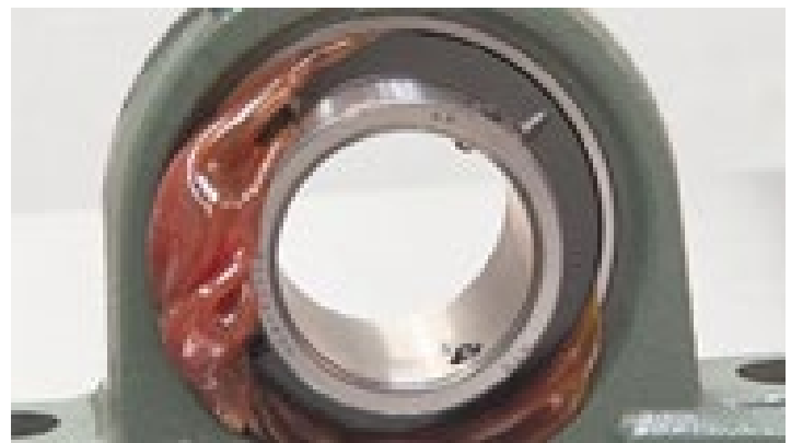
Figure 1: Excess grease purging past lip seals due to over lubrication.
