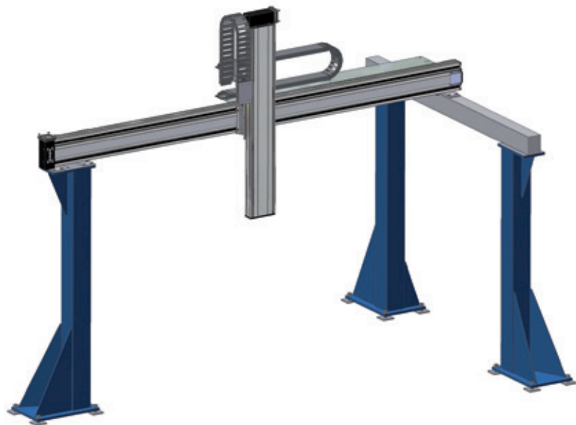
Figure 6.44__ NTN-SNR – Linear Axis system with gantry support legs
