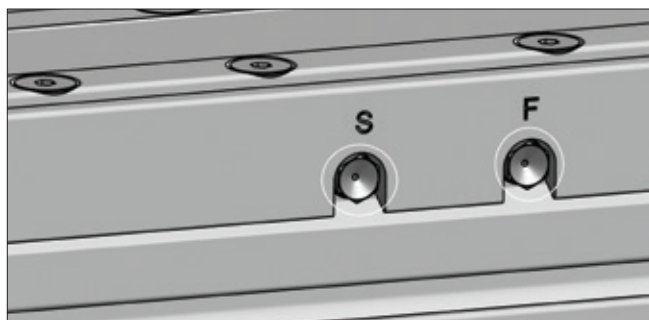
Figure 1.12 __ Slider unit with laterally placed grease nipples
