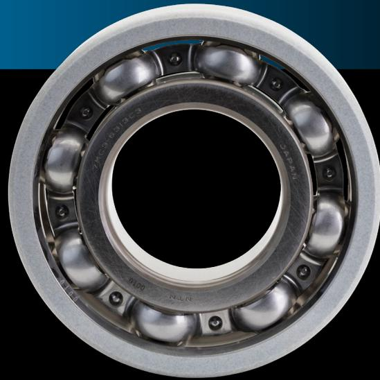
The increase in volume of variable frequency drive (VFD) electric motors as well as other machines where electrical currents are present has demanded the need for insulated bearings. Electrical currents can flow through the bearing causing electrical arcing damage to the rolling contact surfaces, ultimately leading to bearing failure. Electrical pitting and fluting can be prevented with ceramic coated bearings.
